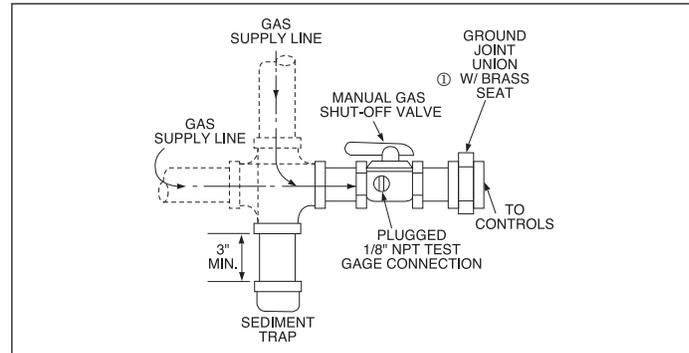
① Manual shut-off valve is in the "OFF" position when handle is perpendicular to pipe.
