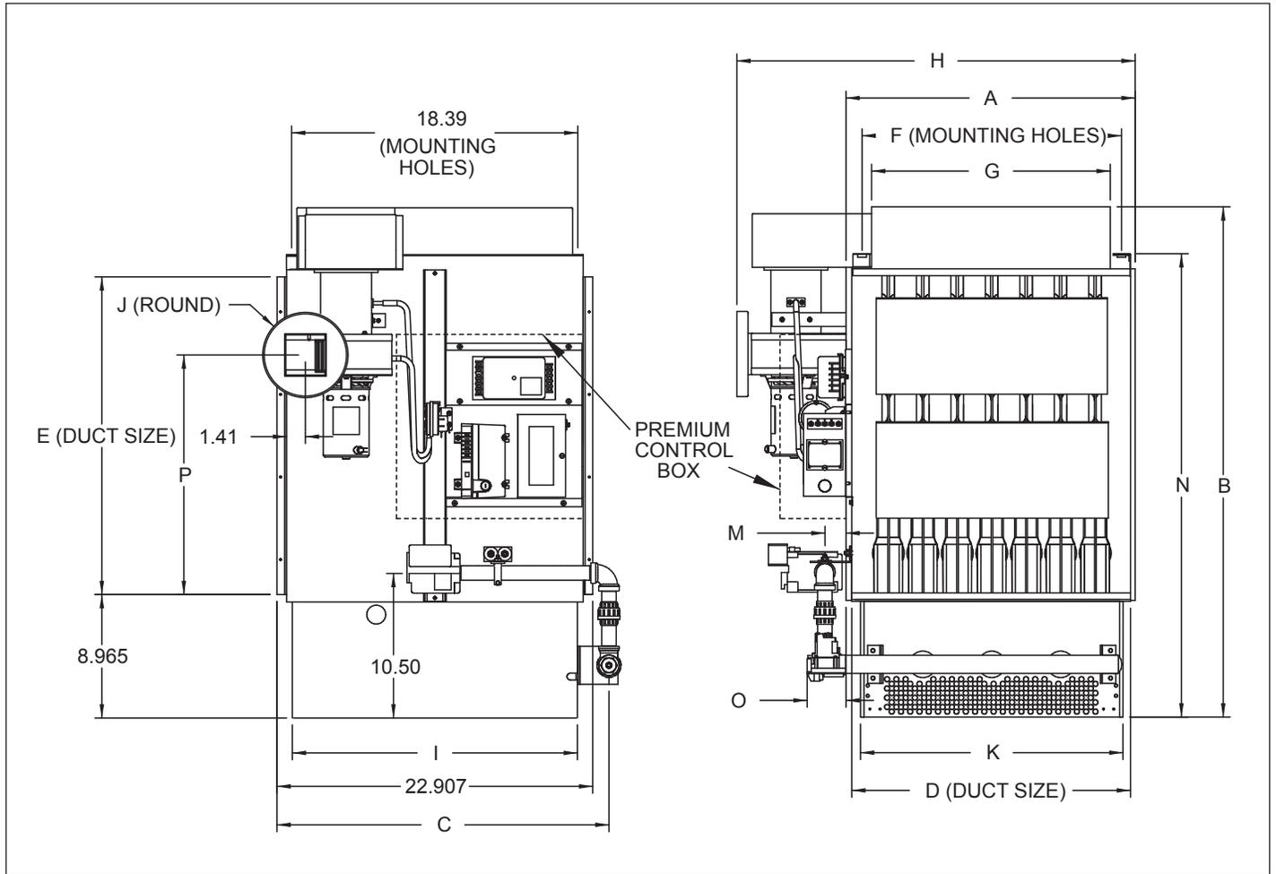
Table 17.1 - Indoor Power Vented Duct Furnace Dimensions
