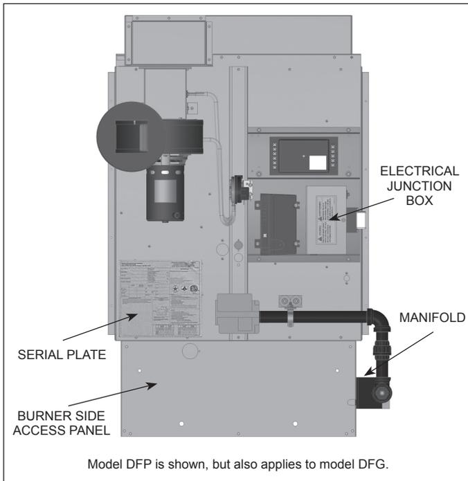
**Figure 19.2 - Burner and Pilot Assembly Removal**
