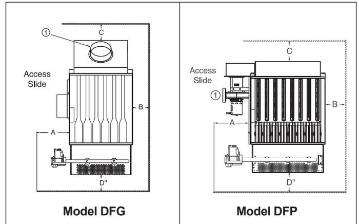
① A 3" minimum clearance to combustible material is required from the vent collar.
